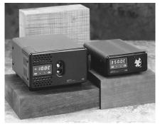
Small enough to fit in your hand, the 9100S comes with any of four block options, each including a different variety of well sizes.
